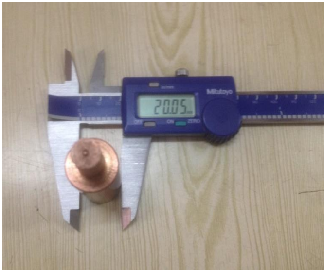
Figure 3. Copper electrode of 20 mm diameter.
