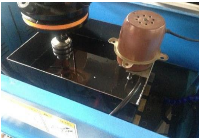
Figure 4. Mid steel tank with 1200 rpm motor
